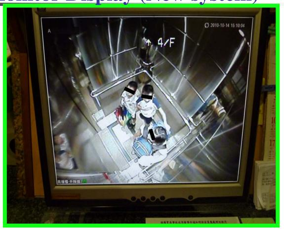
升降機內警鐘按動後 - 影像即時放大至全螢幕顯示 After Activation of Alarm Button inside Lift - Instant "Pop-up" of Full Screen Display
