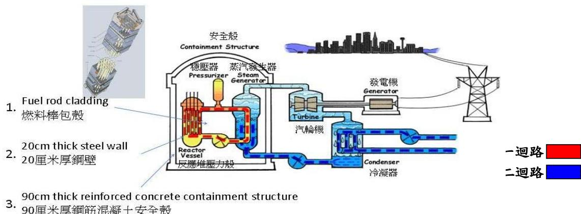
PWR employs a three-barrier design, comprising the fuel rod cladding, a 20 cm steel reactor vessel and a 90 cm thick reinforced concrete containment structure.
