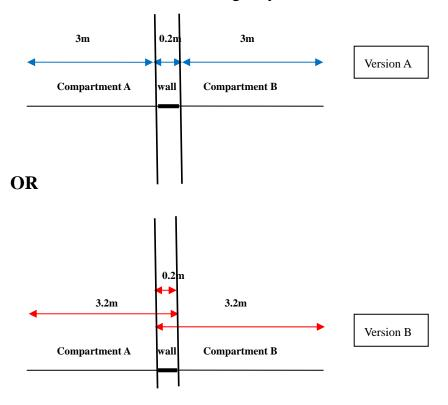
With clear indication, both Version A and Version B show the external dimensions of the two compartments clearly and the issue of "double-counting" will not arise.
