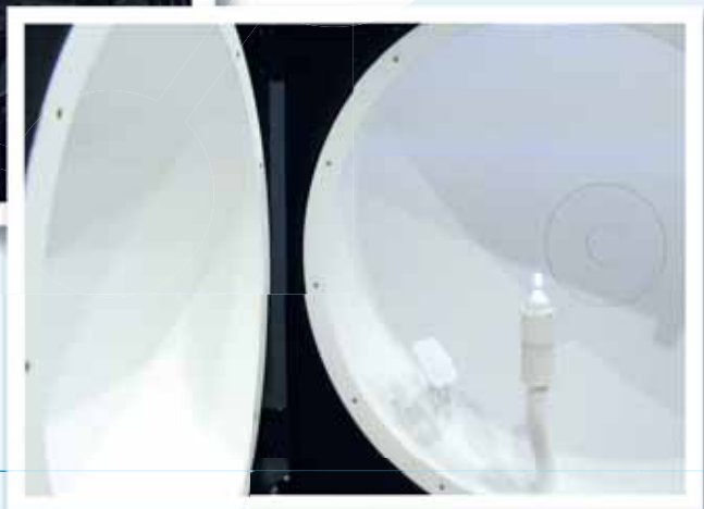
Equipment set-up for testing of an LED lamp in Science Park
