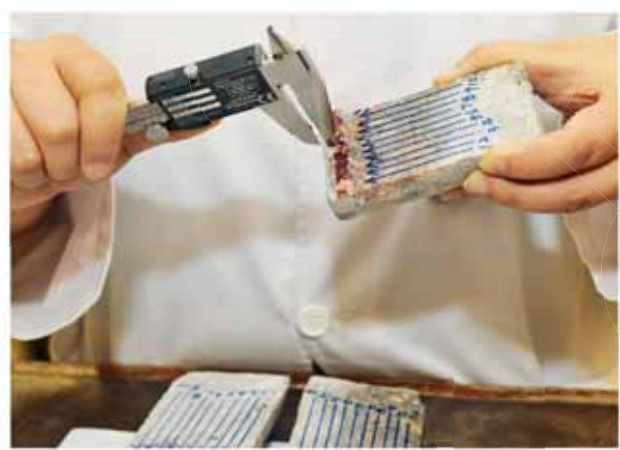
Measurement of carbonation depth in concrete sample
