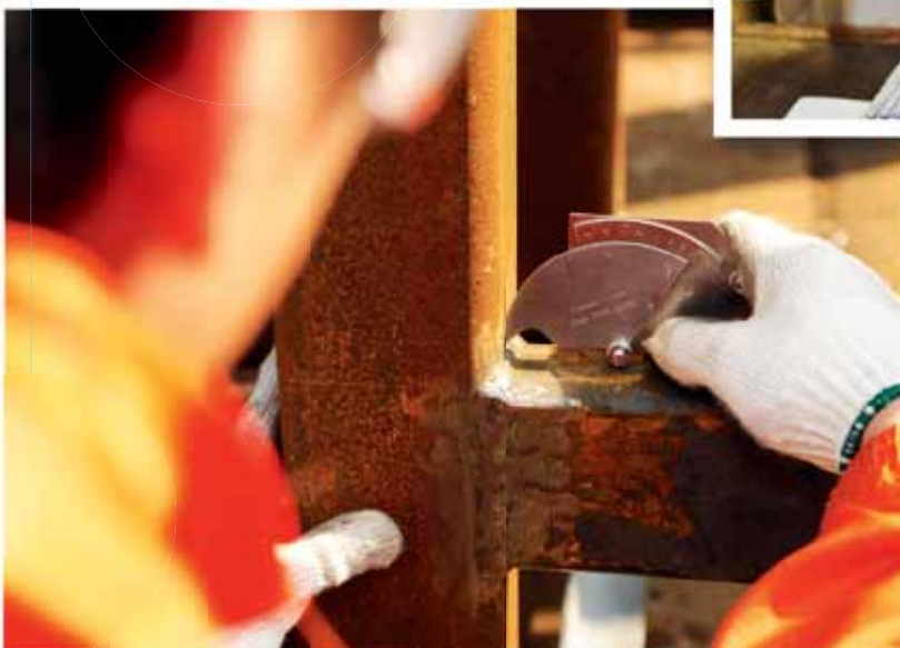
Thickness measurement of weld using weld gauge
