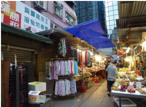
Figure 2.1.4 – Combustible Sunshade of Hawker Stall
