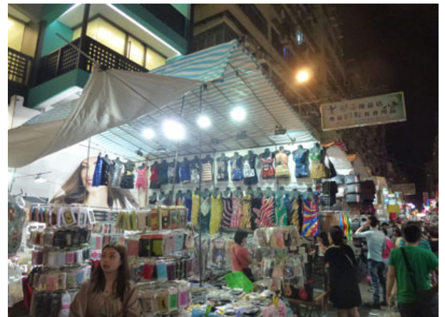
Figure 2.1.7 – Dismantable Hawker Stalls at Tung Choi Street with Combustible Structures
