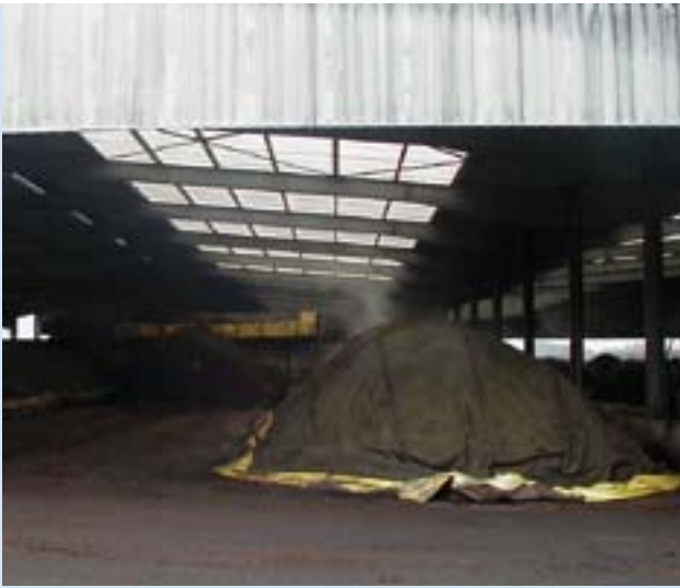
Intensive rotting under a semi-permeable membrane
