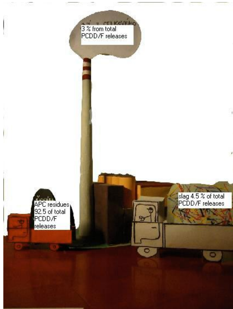
Picture 3: Balance of PCDD/Fs releases into different environment compartments from MWI Liberec.
