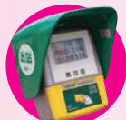
出站收費器 Exit Fare Processor
