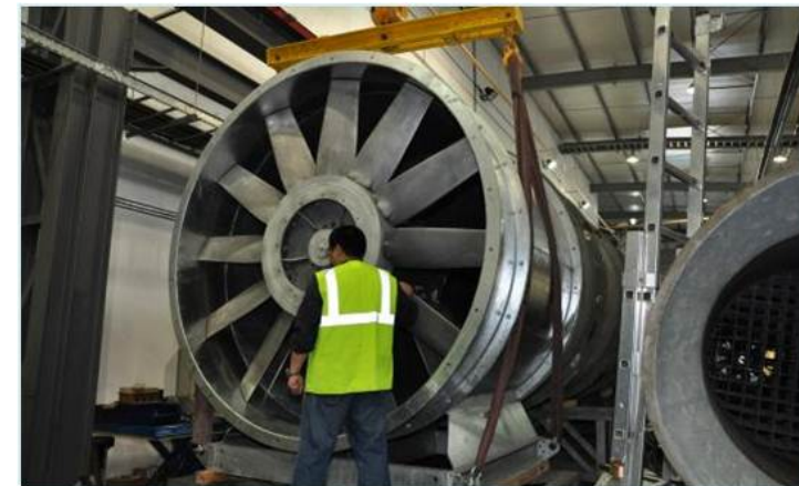
隧道通風風機測試 Factory Acceptance Test for Tunnel Ventilation Fan
