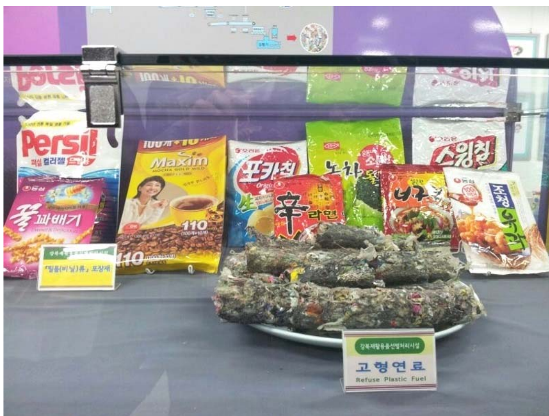
Plastic waste converted into "refuse plastic fuel" for energy production
