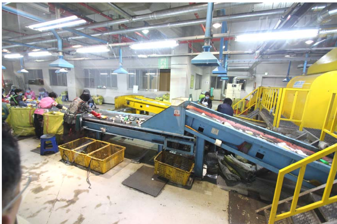
Separation of waste into different categories by workers
