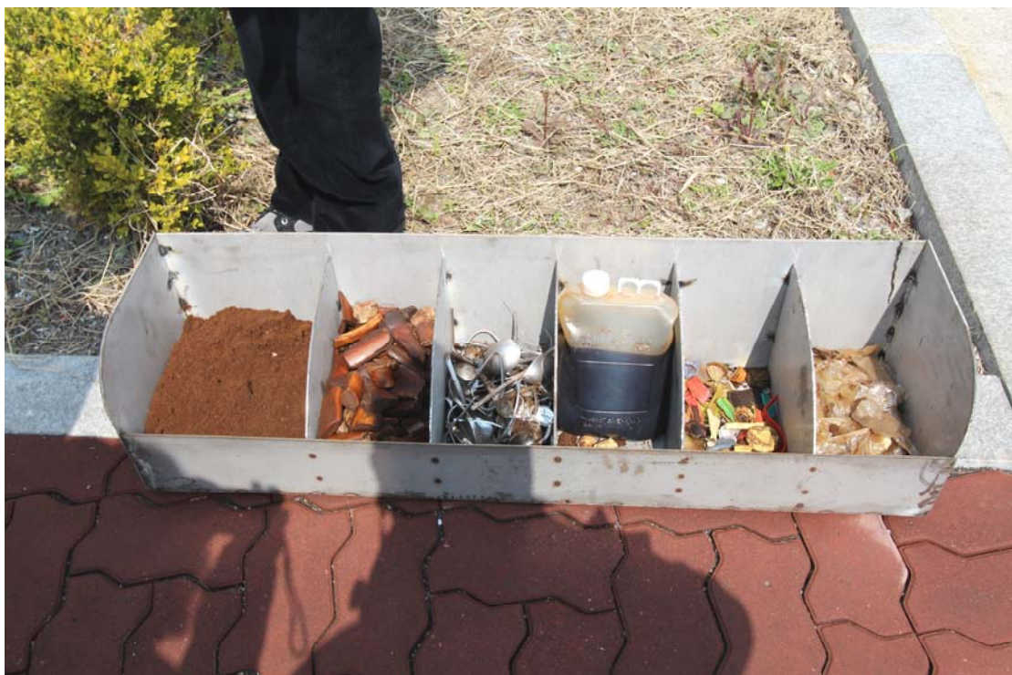
Recycling of food waste into different resources using anaerobic digestion technology. The resultant materials are: (from left) animal feed, bones, steel utensils, biodiesel, recycled residuals, and wooden chips
