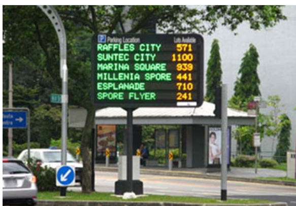
Parking Guidance System (Source: LTA)
