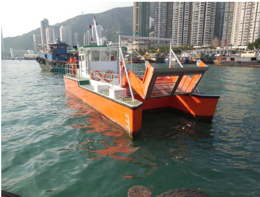
Fiberglass automatic scooper boat, suitable for working at relatively open waters inside Victoria Harbour.
