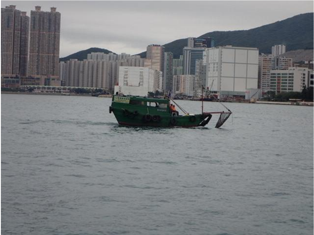
Motor sampan with net, suitable for clearing floating refuse accumulated inside Victoria Harbour and typhoon shelters.
