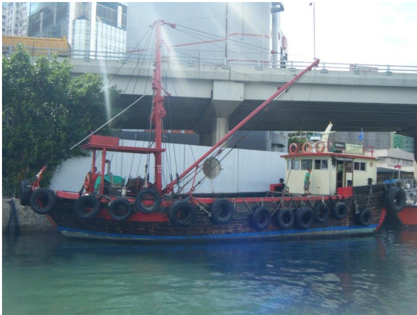
Marine refuse reception vessel used to receive the marine refuse scavenged by motor sampans for onward transfer to marine refuse collection points. It can also be used for handling the heavier marine refuse items.
