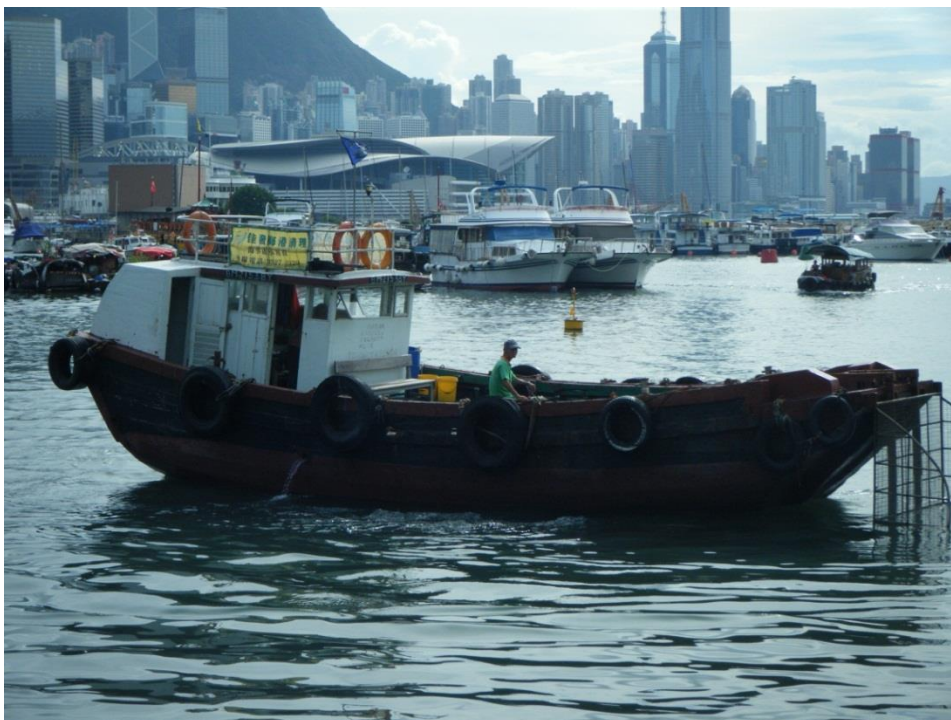
Vessel fitted with motor scooper, suitable for handling the bigger items among marine refuse.
