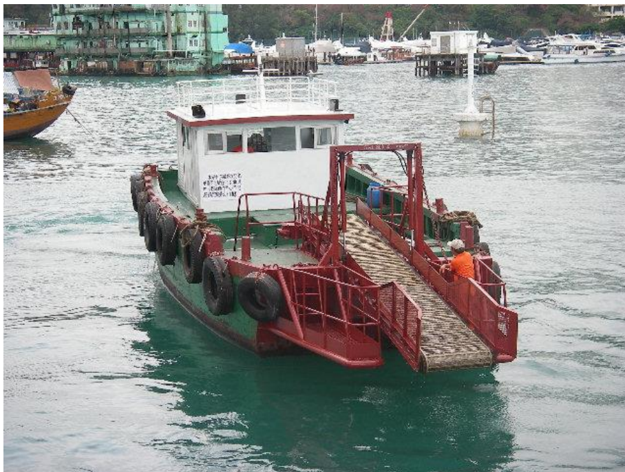
Vessel fitted with marine refuse conveyor belt, suitable to handle a large area of sea surface covered by a large amount of refuse.
