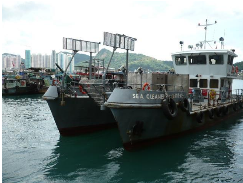
Sea Cleaner Class marine refuse scavenging vessel, suitable for working at off-shore and remote waters.
