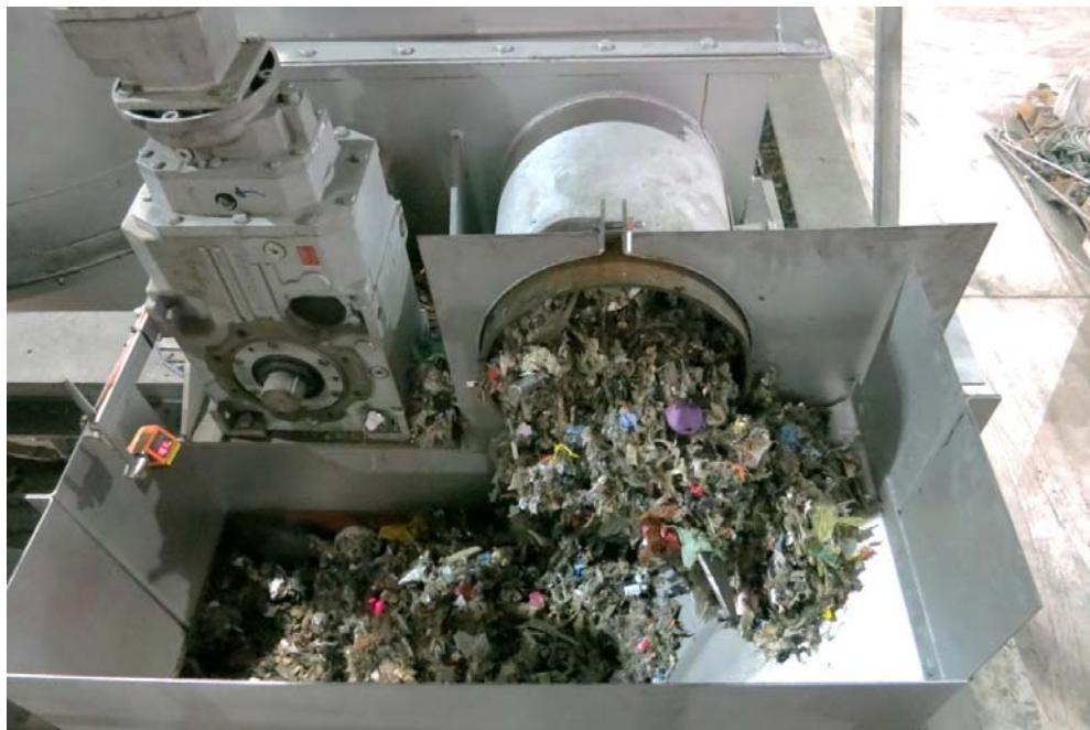
Refuse Derived Fuels were shredded and pelletized to facilitate handling, transportation and storage
