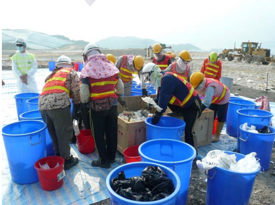
Workmen manually sorting PSBs from a randomly-drawn sample of MSW unloaded from a waste collection vehicle at the South East New Territories Landfill.
