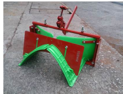
4. Bed shaper To attach behind a tiller or rotavator for forming the shape of the raised soil bed on loosen soil for cultivation.
