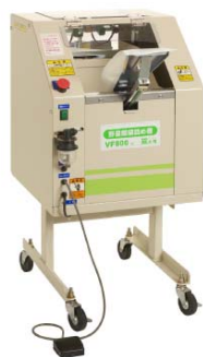
17. Vegetable packaging machine For packaging harvested vegetables.
