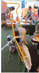
13. Planter For precise seeding directly onto the soil bed.
