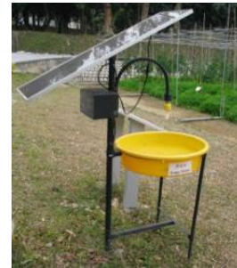
16. Insect attraction lamp To attract insect pests for monitoring and control of pest situation.
