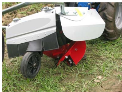
5. Rotary plow To break new ground, building raised bed and creating drainage ditches on harden soil when powered by a tractor.
