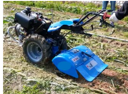
2. Tractor mounted rotavator To break up compact soil into smaller pieces before cultivation.
