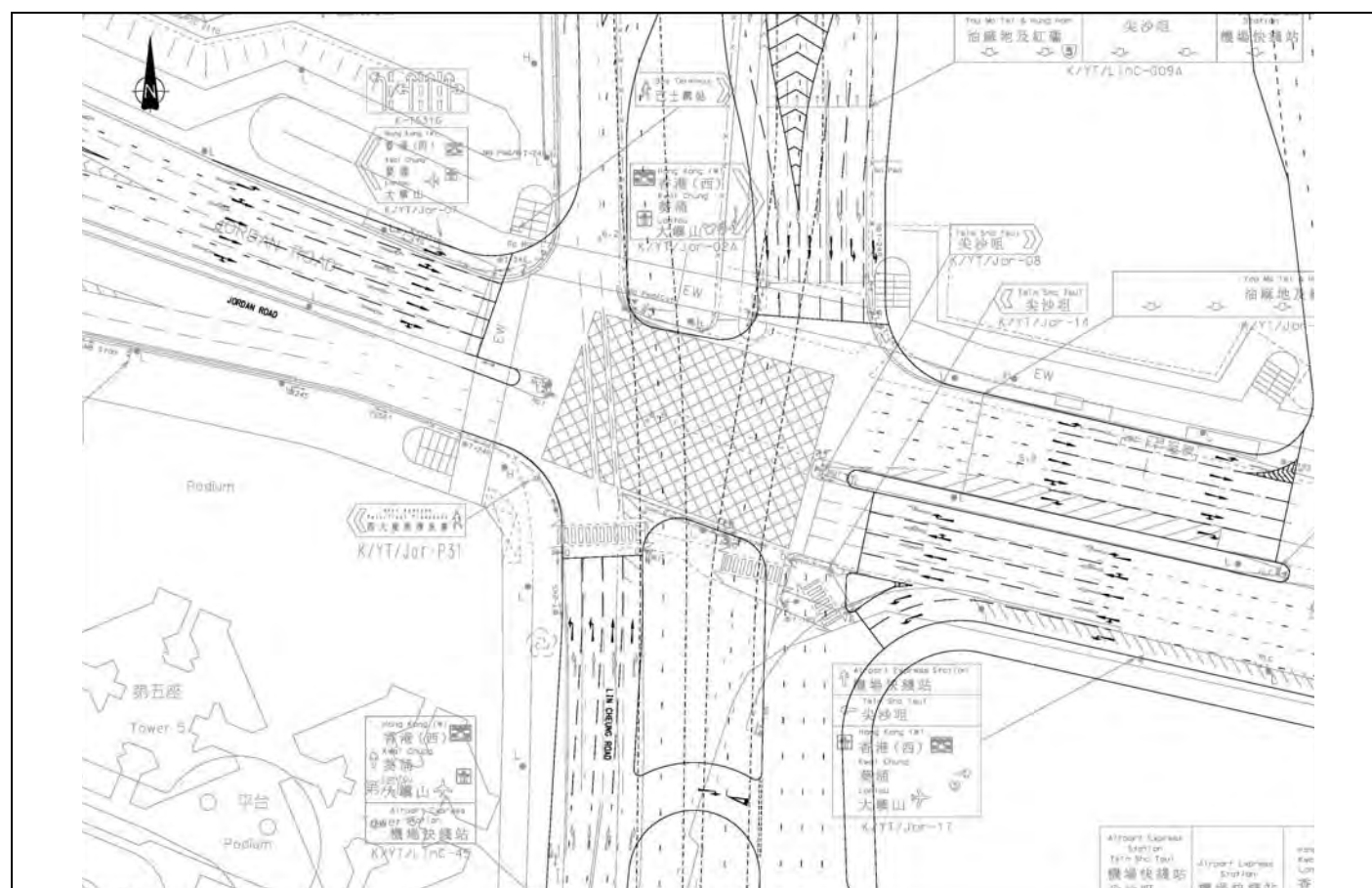
Figure A5 Planned Junction Layout of Lin Cheung Road/Jordan Road (J11)
