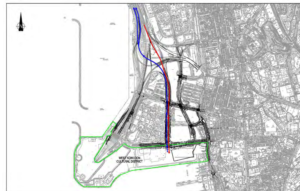
Figure 6.4 Construction Access Points and Traffic Routing for Batches 2+3 Construction Upon Commissioning of LCR-AURW Underpass
