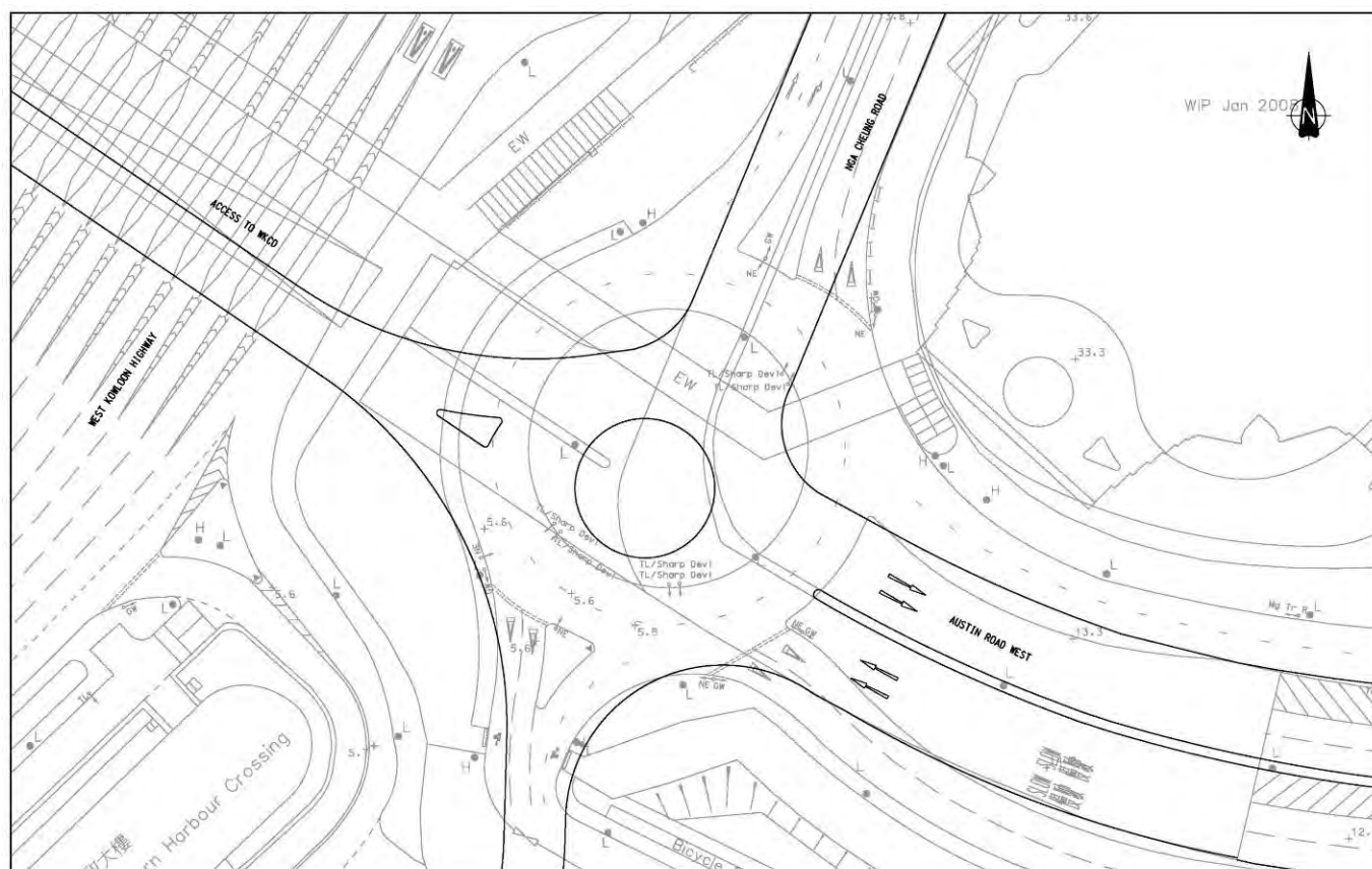
Figure A17 Proposed Junction Layout of Austin Road West/Nga Cheung Road (Elevated) Access to WKCD (WK1)
