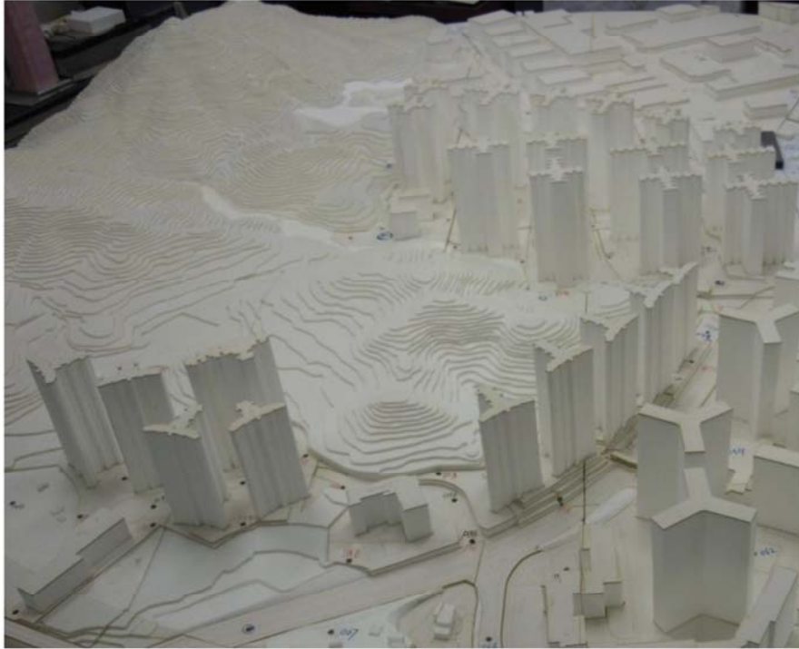
Figure 12. 1:400 scale model for the AVA wind tunnel test. (c) zoomed view of the potential buildings.
