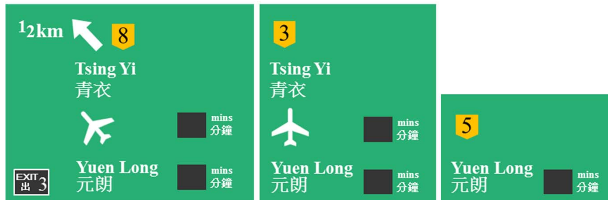
Directional Signs after Addition of Proposed Journey Time Indication System 加設擬議行車時間顯示系統後的交通標誌:
