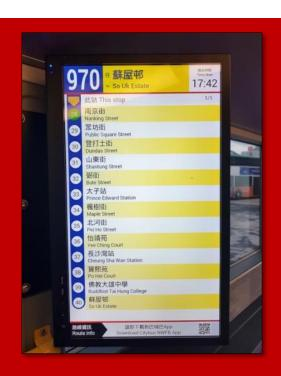
Provide Motion bus stop display panel on most buses 大部份巴士設有動態巴士站顯示屏
