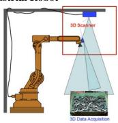
To enhance 3D robotic visual perception, ASTRI has developed a highly accurate and whole-field high-speed 3D scanning technology for robotic eyes which can be deployed in a wide range of applications, including 3D random bin picking, pick-and-place, assembly, navigation, body scanning for garment manufacturing, etc. The underpinning printing, 3D computer vision technology won the Equipment and Machinery Design Award at the 2017 Hong Kong Awards for Industries.
