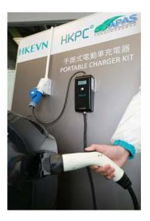
EV PCK separates the traditional EV charger into two parts – socket and charger. The cost to install and maintain a PCK socket is about one tenth of a traditional EV charger, making it affordable to install PCK sockets in car parks.
