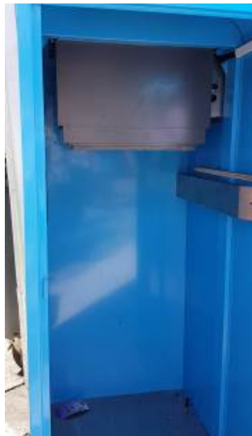
Inner-bin removed showing compactor fully retracted
