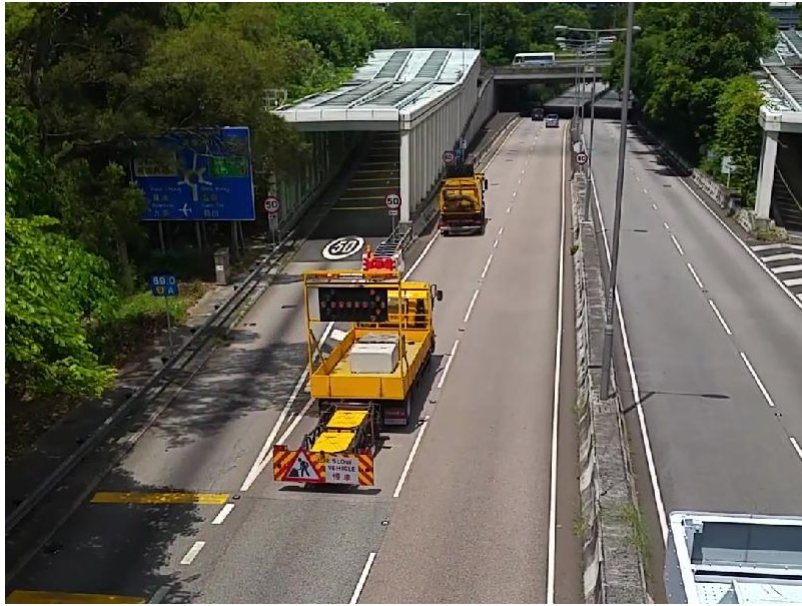
Figure 3 : Escorted by a shadow vehicle with truck-mounted attenuator when conducting mobile operations
