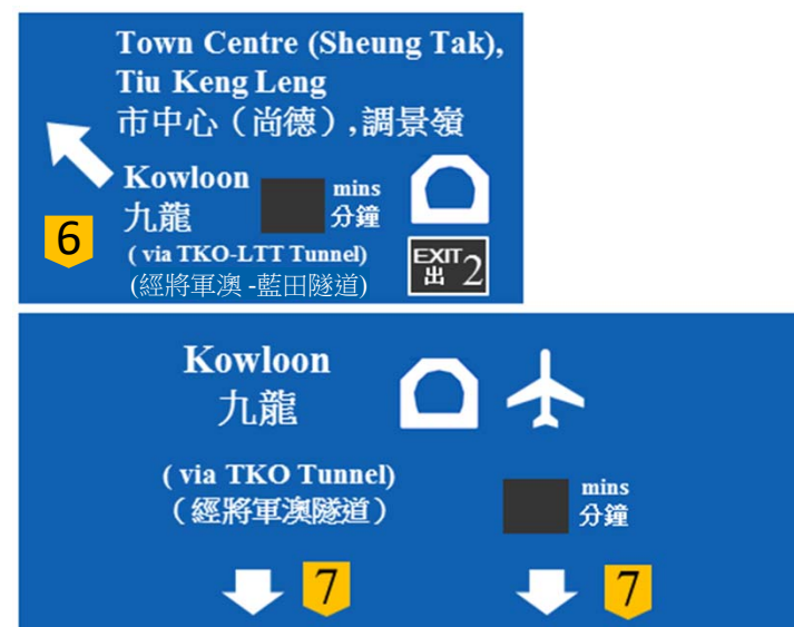
Directional Signs after Addition of Proposed Journey Time Indication System 加設擬議行車時間顯示系統後的交通標誌:
