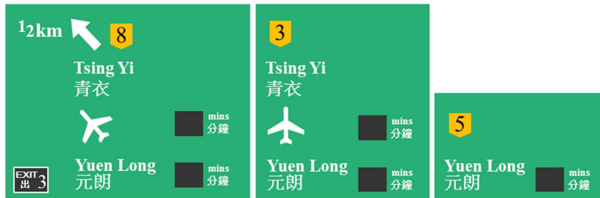
Directional Signs after Addition of Proposed Journey Time Indication System 加設擬議行車時間顯示系統後的交通標誌:
