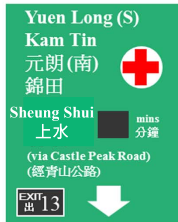
Directional Signs after Addition of Proposed Journey Time Indication System 加設擬議行車時間顯示系統後的交通標誌:
