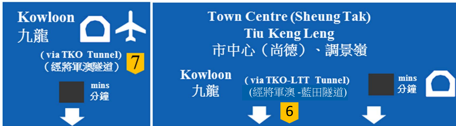
Directional Sign after Addition of Proposed Journey Time Indication System 加設擬議行車時間顯示系統後的交通標誌:
