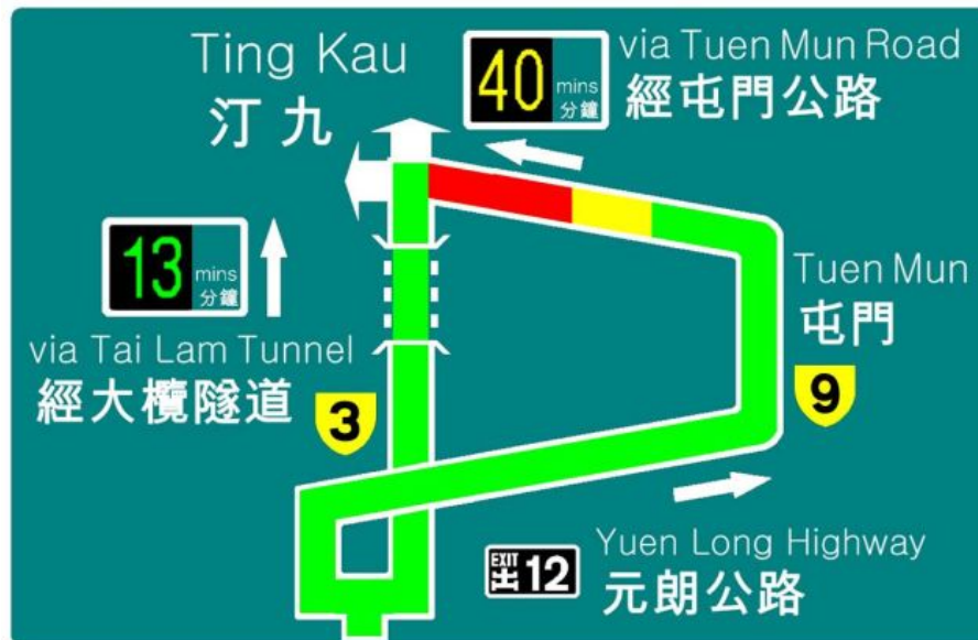
Speed Map Panel at San Tin Highway southbound near Fairview Park 2
