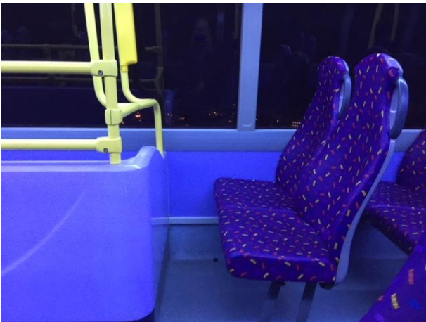
Exposed seats not equipped with seat belts
