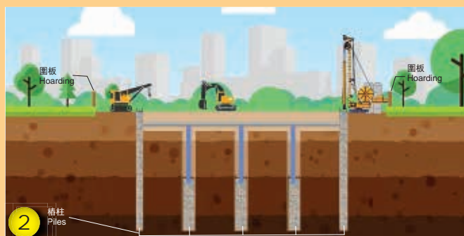
安裝支撐地下空間發展的樁柱及進行地面挖掘以安裝頂層樓板 Install piles for supporting the underground space development and carry out surface excavation for construction of top slab
