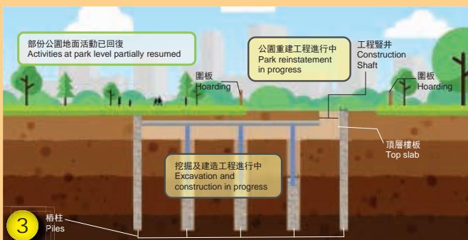
完成頂層樓板後，回填至地面，以儘快還原部分公園設施，並優化公園，讓市民享用 Backfill to surface after construction of the top slab to expedite part of the reinstatement works and facelift the park for public enjoyment
