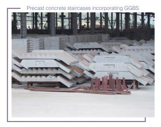
At the level of building materials, we have for some time now made environmentally friendly Ground Granular Blast Furnace Slag (GGBS) part of our specifications for new building contracts. We also require 35% of the cement in concrete used for the construction of precast concrete façades and precast staircases to be replaced with GGBS. This requirement will soon be extended to semi-precast slabs, subject to successful viability studies that are currently underway.
