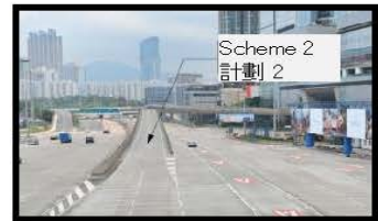
Scheme 2 計劃 2 Proposed single lane elevated road connecting elevated Nga Cheung Road to toll plaza of WHC 擬建高架單線行車道連接雅翔道高架路段至西區海底隧道收費廣場
