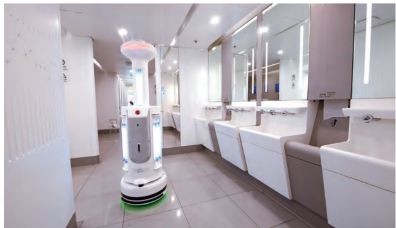
HKIA uses an autonomous, ultraviolet light-equipped robot for sterilisation in the passenger terminals.
