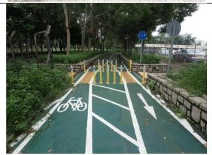
Additional safety facilities at steep ramps to alert the cyclists to slow down and segregate two-way cycling traffic
