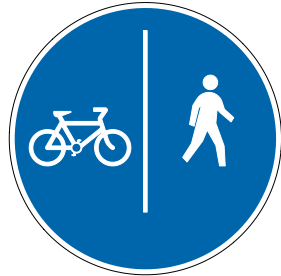
Regulatory signs marking the start of a cycleway, or an adjoining footpath and cycleway
