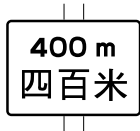
64. Distance as shown to hazard
