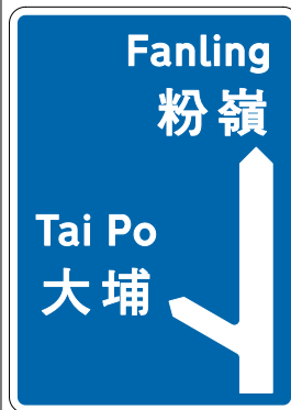
Advance direction sign showing the layout of the junction ahead – the more important the road from the junction, the thicker the line on the sign.
