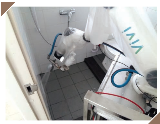
A robot conducting water test at bathroom
