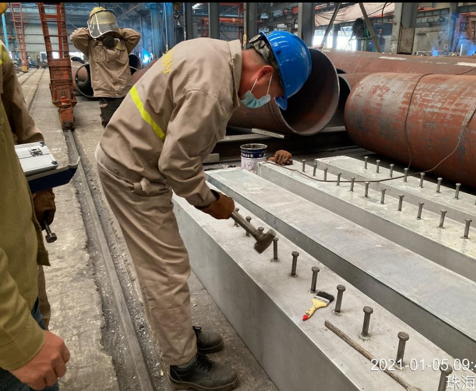
Bending Test to the Shear Studs 剪力釘錘擊彎曲測試
