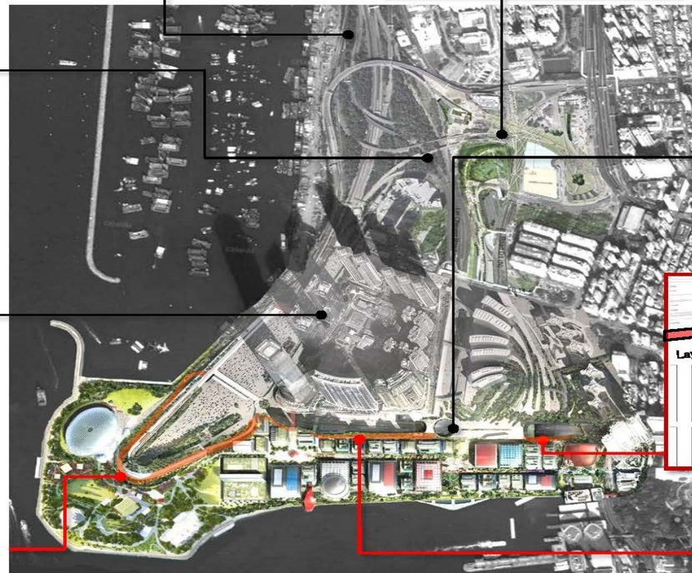
Scheme 2 計劃 2 Proposed single lane elevated road connecting elevated Nga Cheung Road to toll plaza of WHC 擬建高架單線行車道連接雅翔道高架路段至西區海底隧道收費廣場
