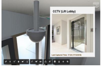
Applying BIM Technology to property management of 618 Shanghai Street for enhancement of work efficiency through remote control of devices and automatic reminders for regular maintenance inspection to upkeep the facilities.
