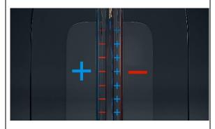
To separate valuable disentangled protein fibres from synthetic textiles materials, this invention is an environmentally friendly system which utilises the triboelectric properties of different kinds of textile fibres to perform the task.
