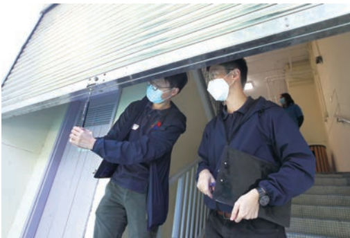
顧問們正使用推拉式張力計以測量拉動捲閘所需的力度。 The consultants used a push-pull tension gauge to measure the force required to pull the roller shutter.
