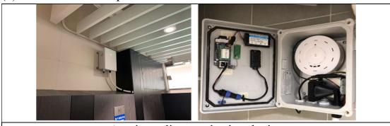
An air quality monitoring device (collecting data on temperature, humidity, odour, etc.)
