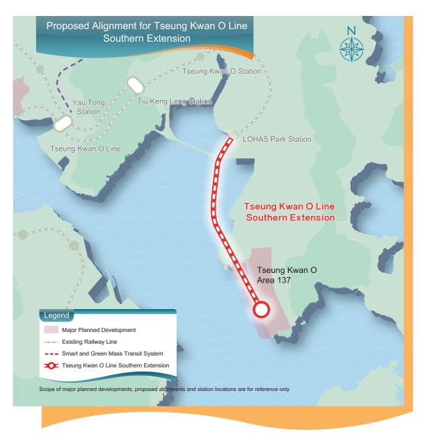
2.4.10 The TKO Line Southern Extension, spanning approximately 4 km, aims to support the development of TKO Area 137 and provide a convenient and efficient mass transit system to the 135 000 new population. The Government recommends using the heavy rail system of the existing TKO Line as the basis, and extending the railway from the at-grade LOHAS Park Station southward to the underground station at TKO Area 137 via tunnels through the seabed
