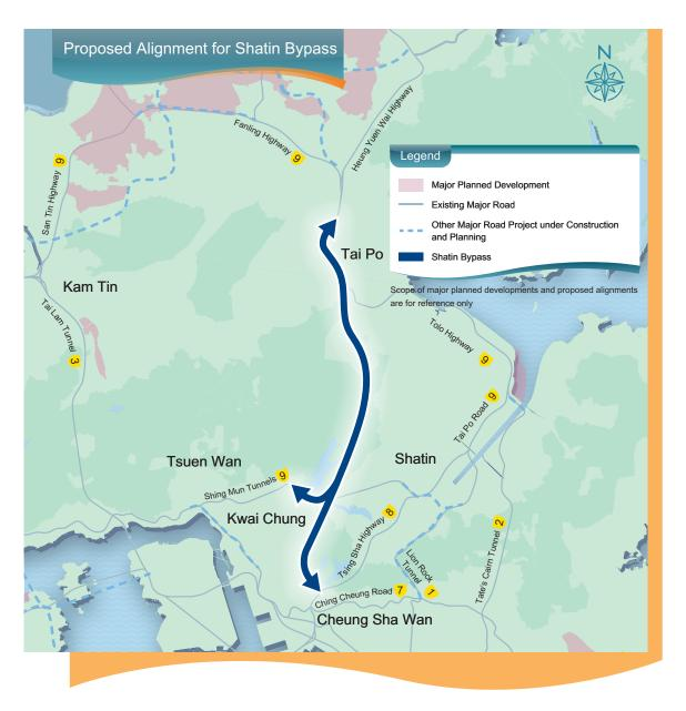
**2.4.18** The Shatin Bypass is approximately 15 km long. Compared with the existing Tolo Highway and the Tai Po Road, the Shatin Bypass will serve as a more direct north-south corridor, connecting the northeast New Territories with the urban areas of Kowloon. Its northern end will connect to the Fanling Highway in Tai Po, providing convenience not only for road users in the North District but also for residents in Tai Po, Tai Wo, Hong Lok Yuen, Lam Tsuen
