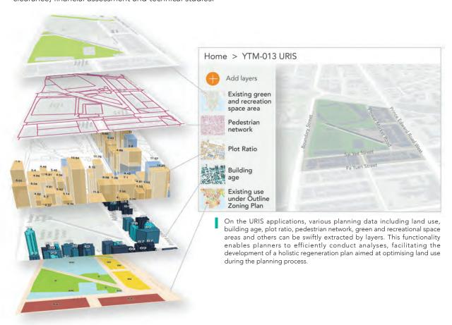
Since 2021, we have also been utilising Three-Dimensional Intelligent Map (3D iMap) technology for the freezing survey conducted at the onset of our redevelopment projects. This technology provides real-time, on-site monitoring of survey progress and helps us deploy manpower more efficiently. We also analyse the living status and demographic data of households via the 3D iMap to expedite future acquisition and rehousing efforts.
