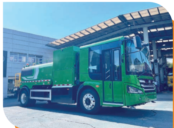
Hydrogen fuel cell street washing vehicle
