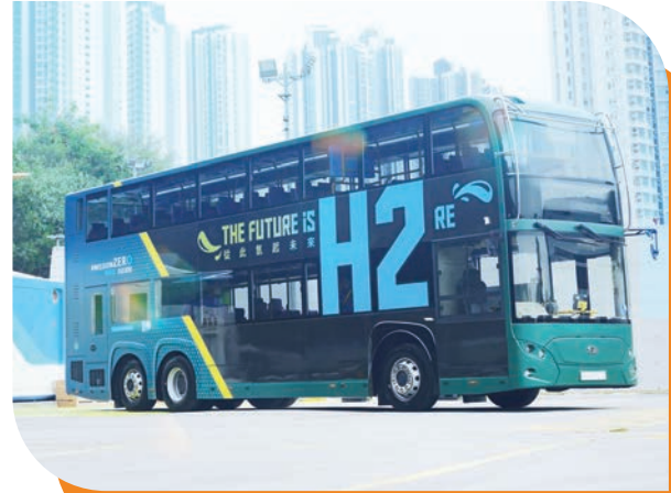
The world's first tri-axle HFC double-deck bus
