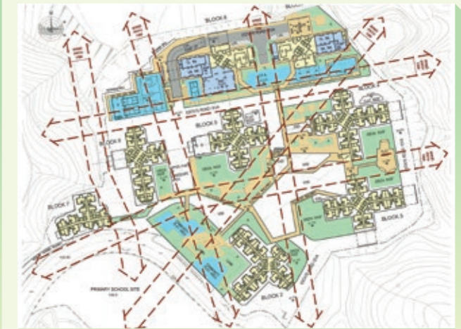
大埔富蝶邨善用布局，在住宅大廈間留下通風走廊，加強自然通風 The domestic blocks at Fu Tip Estate, Tai Po are positioned to form open breezeways for better natural ventilation
