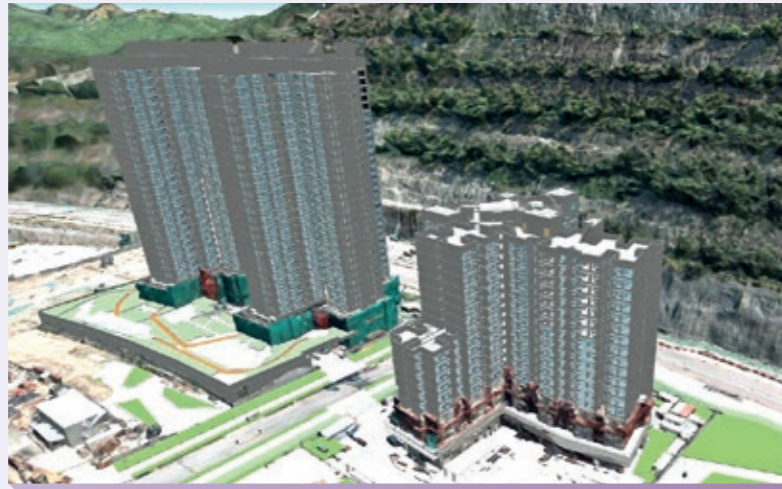
「智築目」監察預製組件由生產至安裝的進度（左圖）及其三維視像化資訊 HA-PIMAP monitors the status of precast units from production to installation (left photo), and its 3D visualisation
