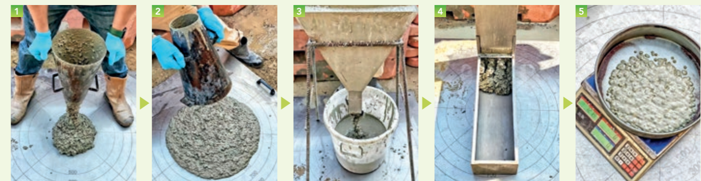
我們的合作研發機構在先導計劃的試驗樁應用粒化高爐礦渣粉前，就不同配比的礦渣粉混凝土配方進行測試（左起） Our collaborative research institute conducted tests on different GGBS concrete formulations (from left) before applying GGBS to the test piles of a pilot project
